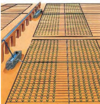
Zero Energy Micro Irrigation System on flat land
