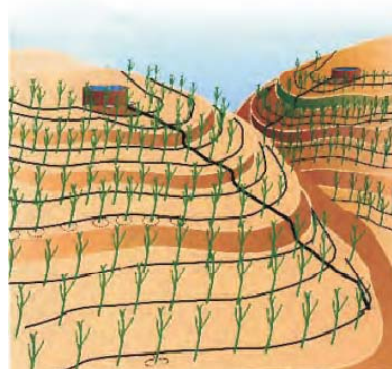
Zero Energy Micro Irrigation System on undulating land.
