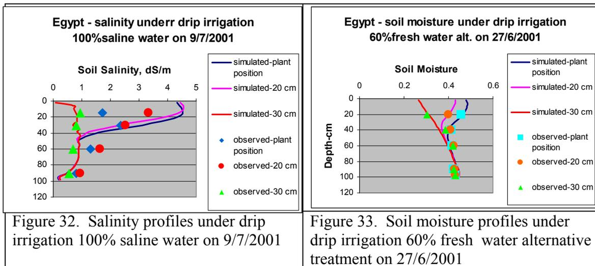
Figure 32. Salinity profiles under drip irrigation 100% saline water on 9/7/2001
