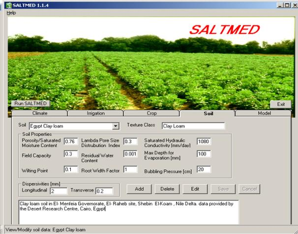
Figure 2. Soil parameters used in the calibration of Egypt 100% fresh water treatment, 2002 season.
