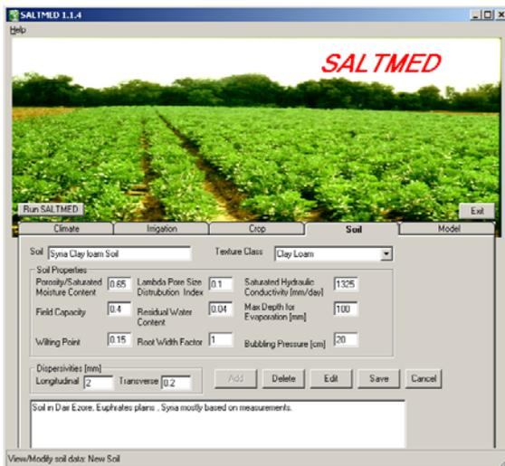
Figure 8. Soil parameters used in the calibration of Syria 100% fresh water treatment, 2002 season.
