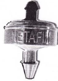
**Figure 23.** A kind of dripper is self cleaning, antisuction mechanism, compensating in 0.7 to 4 bar range. At 0.12 bars opening is closed toward reverse flow into dripper.
