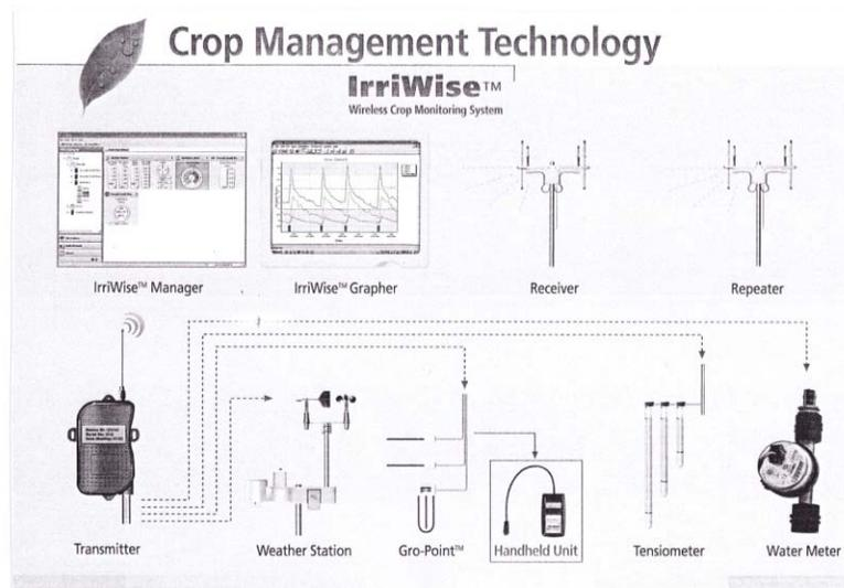
**Figure 10.** Components of a wireless crop monitoring system
