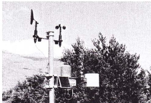
**Figure 1.** Automated intelligent meteo operation in field, Karaj- Iran
