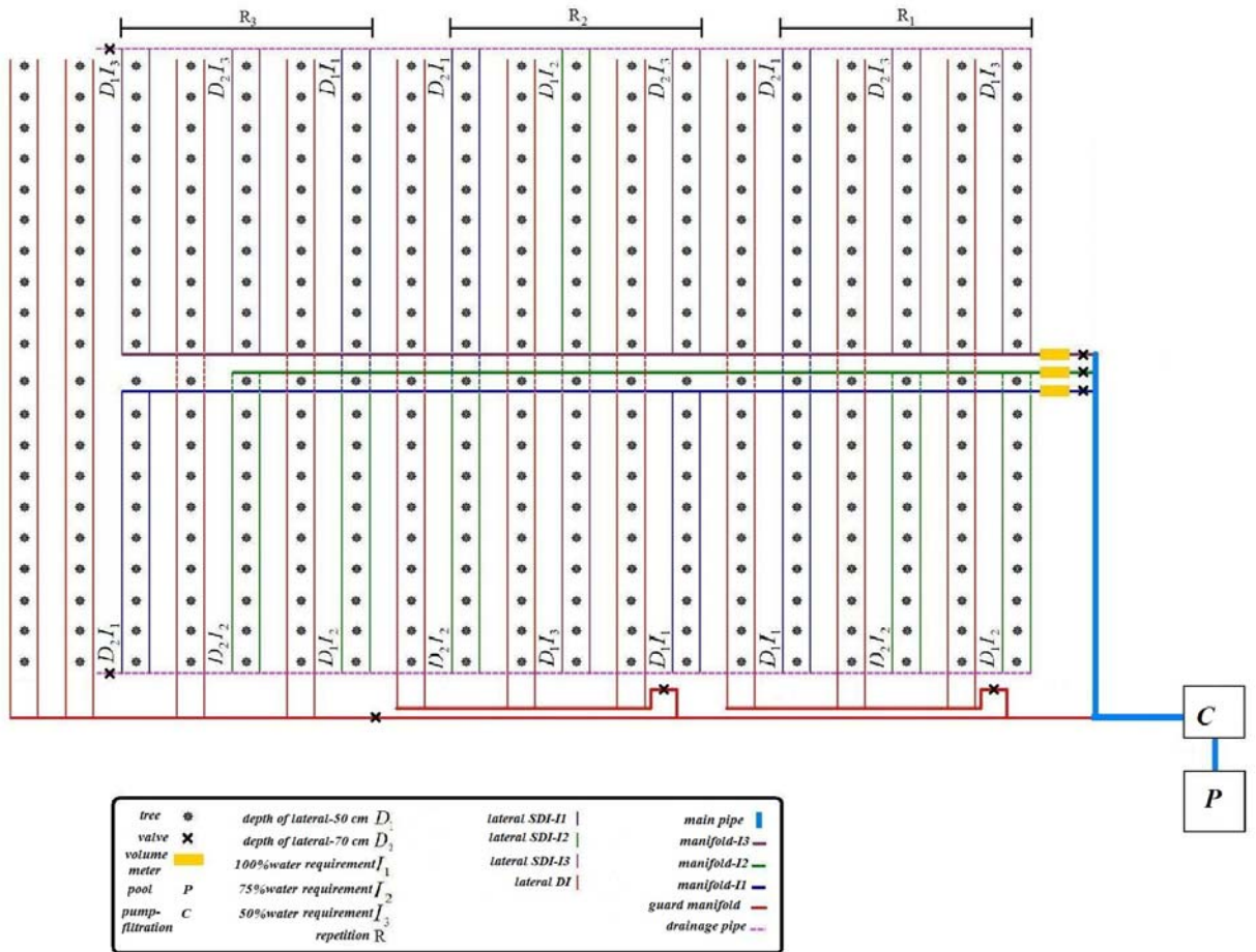
Figure 1. Schematic description of saline-water use experiment under drip irrigation in the pistachio orchard.
