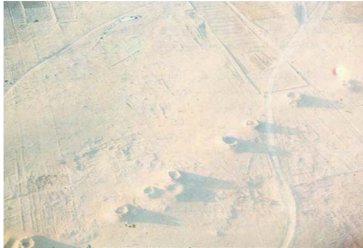
Figure 151 , This photograph shows the piles of dirt around the mouth of shafts, taken from the air. These piles form a perspective showing the direction of a Qanat on the surface.
